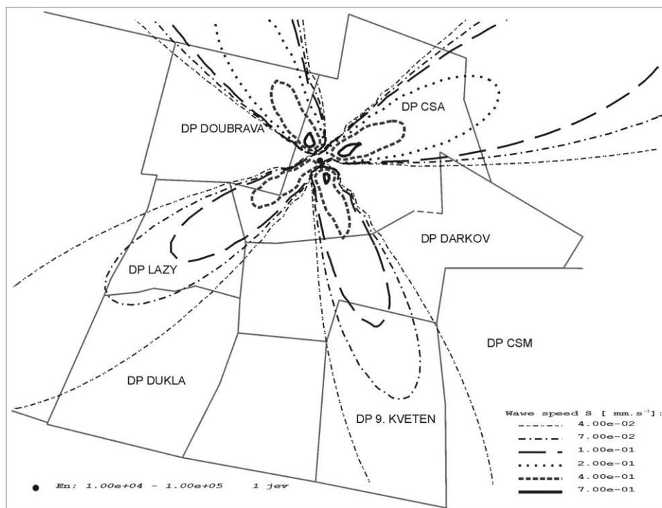
Fig. 3.2. Map of isolines of ground velocity (values of isolines were optimized by computer program) for mining tremor on 18.6.2005, which epicenter was located in the area of CSA Mine
