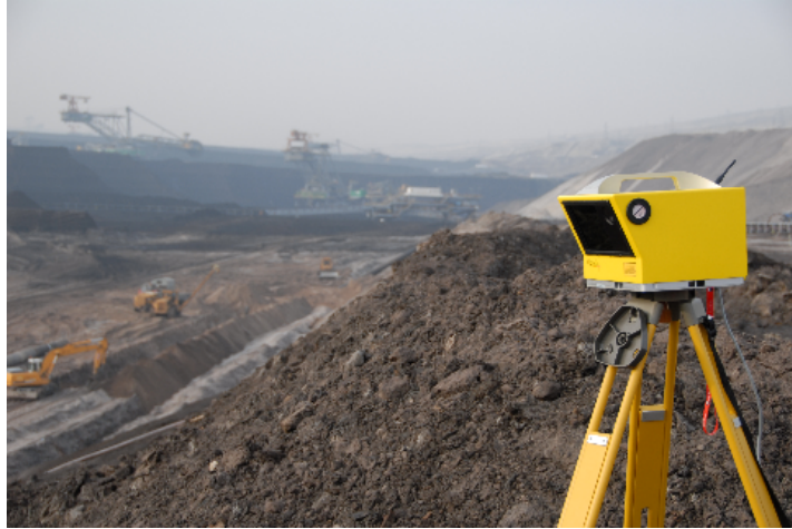
Rys. 2.1. Skaner ILRIS 3D podczas skanowania osuwiska Fig. 2.1. Scanner ILRIS 3D during the scanning of the landslide
