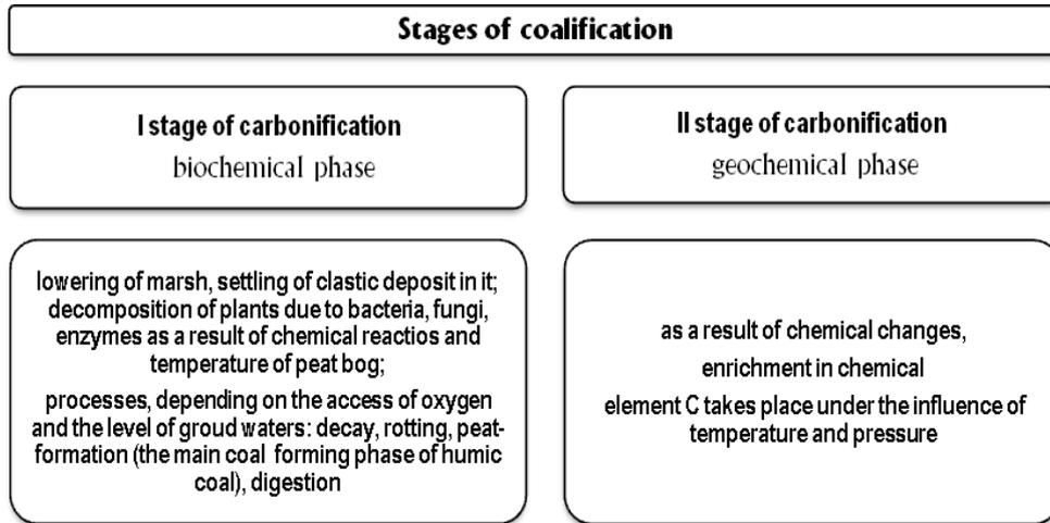
Fig. 1.1. Stages of coalification of coal generating organic matter
