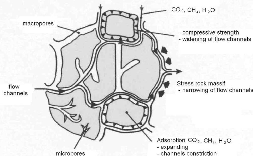
**Fig. 2.2.** Model of porous structure of coal and some factors which influence it (Seewald, Klein 1985)
