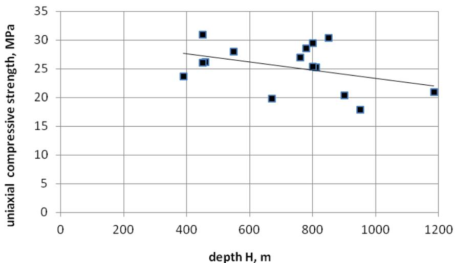
**Fig. 3.6.** Relation between compressive strength of semi-bright coal and deposition depth in the USCB (Bukowska 2012)
