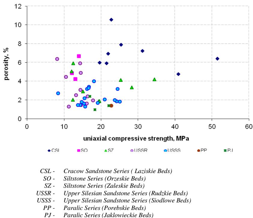
**Fig. 2.6.** Relations between coal porosity and compressive strength
