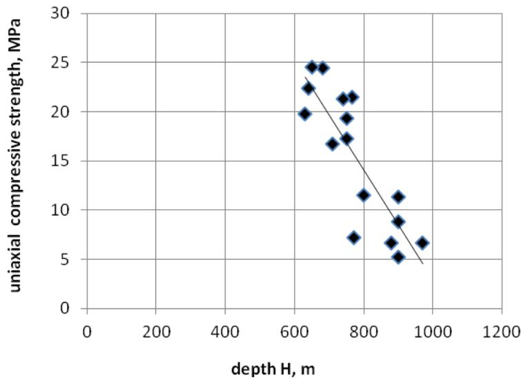
**Fig. 3.5.** Relation between compressive strength of bright coal and the depth of current exploitation in the USCБ (Bukowska 2012)
