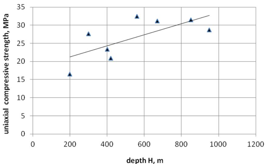
**Fig. 3.7.** Relation between compressive strength of semi-bright coal with interbedding of dull coal and deposition depth in the USCB (Bukowska 2012)
