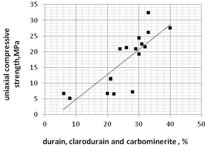
**Fig. 3.4.** Relation between compressive strength and fraction of the most resistant microlitotypes of hard coal in the USCБ (Bukowska 2012)
